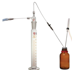
Fig. 12 Double-tipped needle transfer to graduated cylinder
