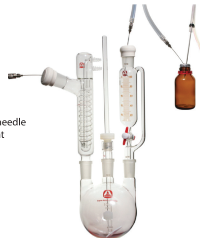
Fig. 13 Double-ended needle transfer with syringe valve
