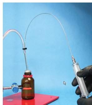
Fig. 8 Filling syringe using nitrogen pressure
