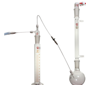
Fig. 13 Double-ended needle transfer with syringe valve
