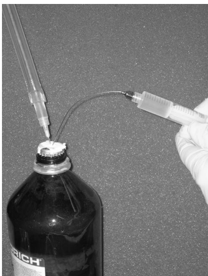
Fig. 3 Inert gas bubbles and excess liquid are forced back into reagent bottle
